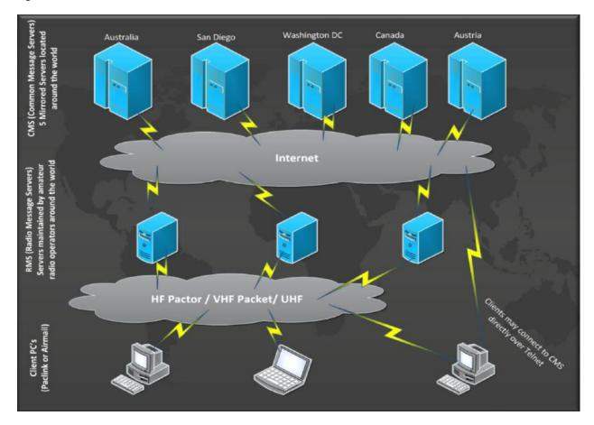
The Winlink system consists of a group of Common Message Servers (CMS) placed at various locations around the world. These servers connect via the Internet to Radio Message Servers (RMS) in many geographic locations to form a star network configuration. The Radio Message Servers are the VHF, UHF, or HF RF gateway into the Winlink system. The final component is
